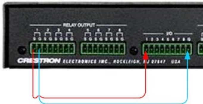
Figure 8 - CP4-R Relay Wiring
